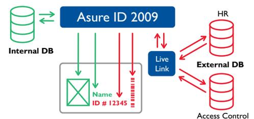
**Live Link real time data exchange** lets you mix cardholder data from internal and external sources on the same card. The Live Link Wizard simplifies setting up connections to external databases.
